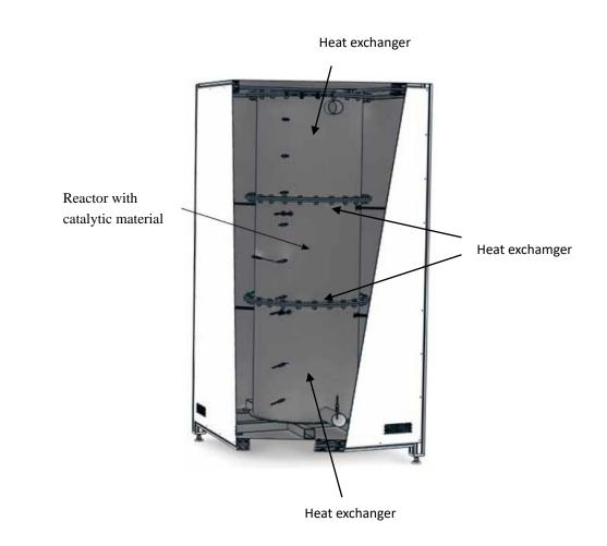
High performance isolation material is used to minimize heat loss from the reactor module. A number of temperature sensors is mounted in the reactor module for temperature control.
