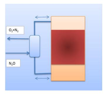
The gas flow is periodically being switched using pneumatical dampers.
