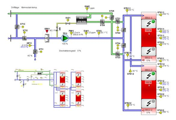
When the gas flow change direction there is also a switch of the active heater.
